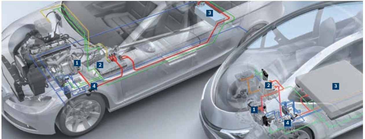
Left: Parallel full hybrid with electric motor – between internal combustion engine and transmission – integrated into the drive train Right: Electric vehicle with electric drive for the front axle
