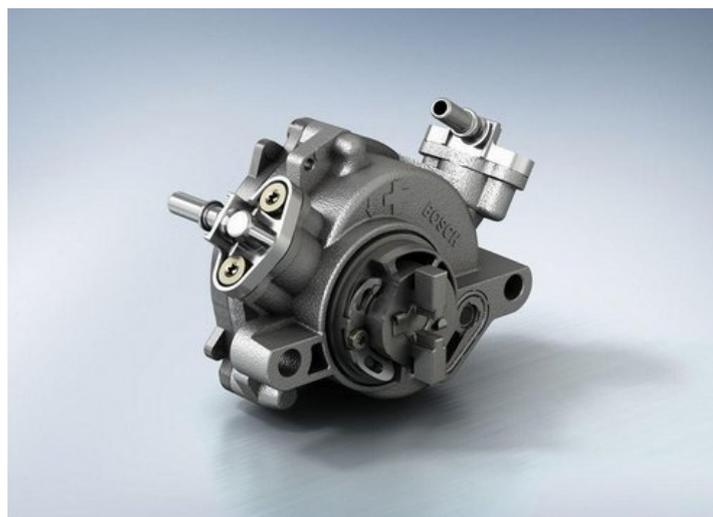
To achieve this advance, Bosch completely redesigned this time-tested component, which has been produced 45 million times to date: the new generation is 300 grams lighter than other mechanical vacuum pumps and even more than one kilogram lighter than electric vacuum pumps. A thermoplastic rotor makes the difference. Its dimensionally stable vanes generate the needed vacuum, but the rotor weighs considerably less.
