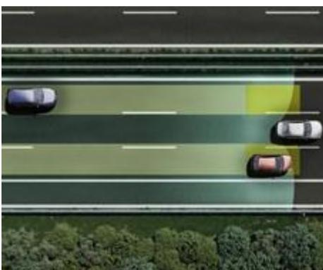
The lane change assistant can prevent hazardous situations when changing lanes and thereby reduce the risk of an accident. The system is based on two midrange radar sensors in the rear of the vehicle that monitor the areas next to and at an angle behind the vehicle.
