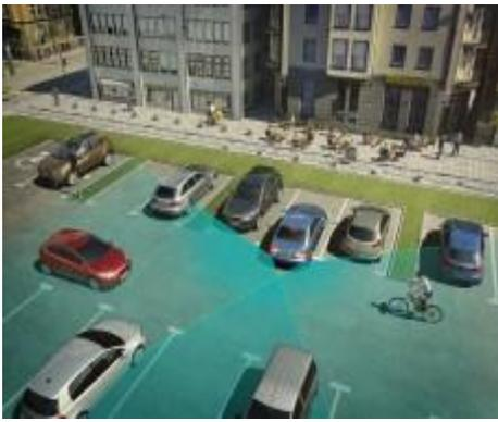
Backing out of a parking space at a right angle to the traffic lane can be especially challenging, particularly when the driver is unable to see cross traffic behind his own vehicle, for example because his vision is blocked. The cross traffic warning makes it easier to back out of right angle parking spaces.
