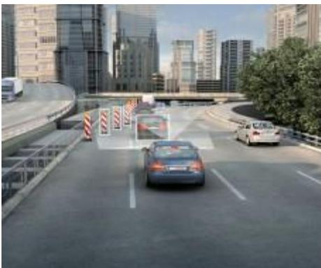
The construction site assistant is an expansion of the lane assist program, including for narrow highway construction sites. It is based on a stereo video camera and is active at speeds up to 100 km/h. In narrow lanes, the function helps the driver maintain a safe distance between vehicles in the adjacent lane and safety curbs and guard rails.
