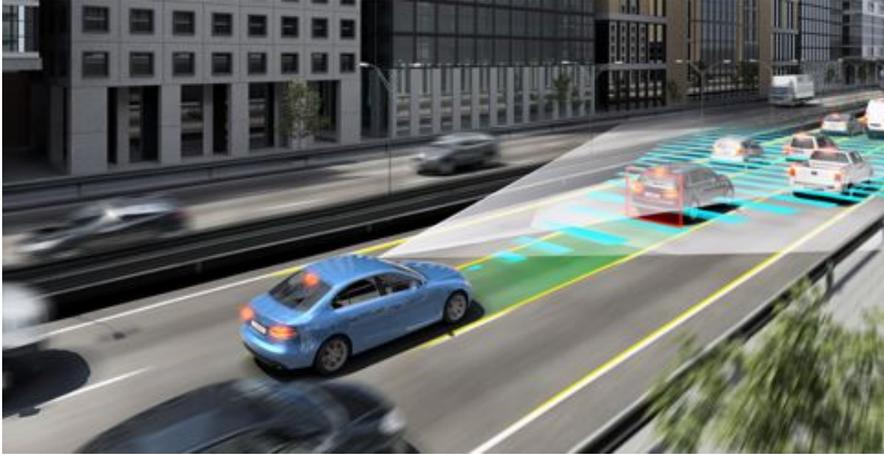
In the fusion of sensor data, the advantages of physically different sensors or ways of measurement are optimally combined to yield information that individual, isolated sensors are incapable of providing. The fusion of several sensors increases the measuring range, and enhances measurement reliability as well as precision. The difference measuring principles are also used to confirm individual objects.
