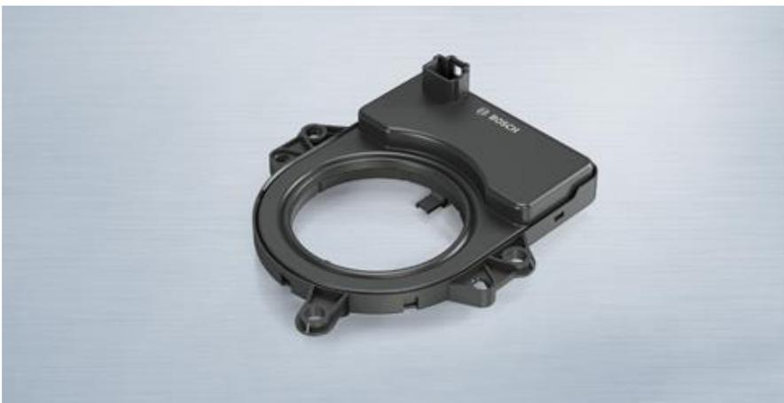
The steering angle sensor detects the position of the steering wheel by determining the steering angle. From the steering angle, speed and desired braking pressure or position of the accelerator, the driving maneuver desired by the driver can be calculated.
