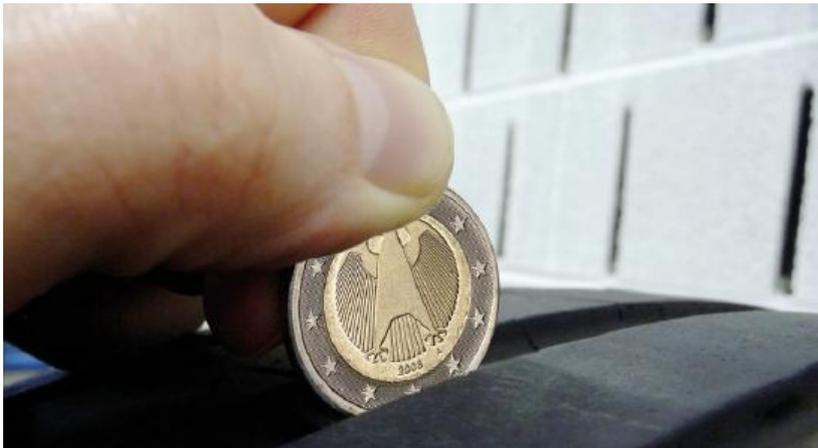
The ring of stars is visible in this case and the tires should be replaced.
