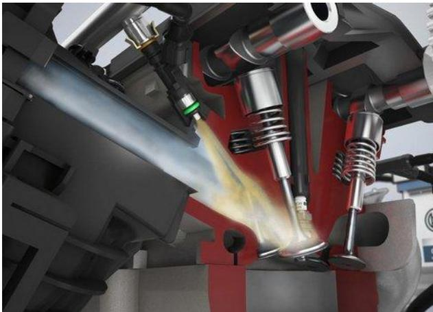
Advanced port fuel injection: Bosch has developed four individual approaches to improving gasoline port-fuel injection. This cost-effective systems approach can reduce fuel consumption by as much as 12 percent. In addition, advanced port fuel injection (advanced PFI) can improve torque and engine performance. Using this system, therefore, drivers can reduce fuel costs while experiencing greater driving enjoyment at the same time.
