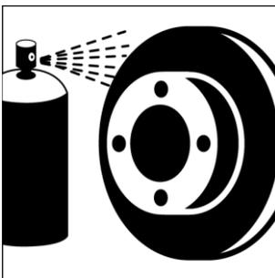
Long-term corrosion protection is provided by brake disks supplied with aluminium or zinc dust coating.
