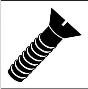
Use should always be made of new bolts on replacing brake disks. This symbol on the pack indicates that the bolts are included in the scope of delivery. The bolts for these brake disks do not have to be ordered separately, thus saving time.
