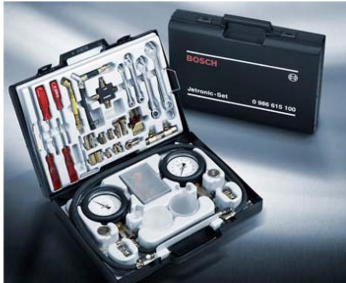
In addition to a 16-piece tool kit with diverse combination wrenches and screwdrivers, the set also contains CO adjustment tools (for various BMW vehicles), hose clamps, hoses, adapters, connection parts, valves, plug-in nipples, seal sets and two pressure gauges (0 to 10 bar and -1 to 1.5 bar). All hoses are equipped with a plug-in system to ensure fast, secure and problem-free connection.
