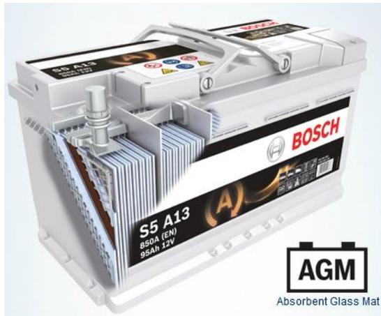
AGM batteries are regarded as the best lead-acid technology in the market: They have a particularly high current capacity and at the same time a high deep-cycle resistance. (Standard lead batteries are optimized for only one of these factors!) Typical use: Passenger cars with start/stop system and regenerative braking.
