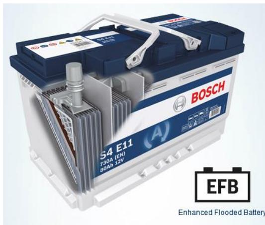
In terms of their deep-cycle resistance and their insensitivity to electrolyte stratification, EFB batteries are located somewhere between standard batteries and AGM batteries. They are, however, not equipped with fiberglass mats and VRLA (valve-regulated lead-acid) safety valves. Typical use: Passenger cars with start/stop function and regenerative braking.
